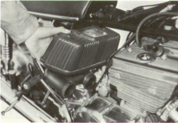
Fig. 7-1-13 Removing air cleaner
