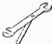
Point wrench with 0.35mm gauge
